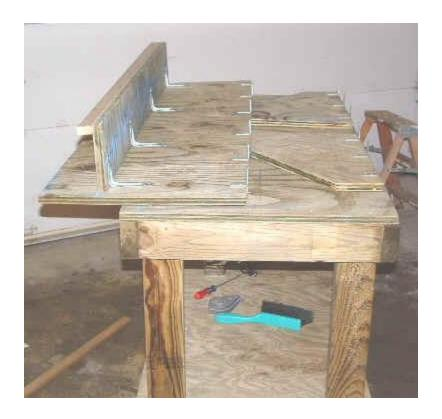
Now mount the top shelf to the back of the potting bench using the line that you have already drawn as a guide. The wood screws you use in this step should only be 3/4" long, and even then you might have to file off the points so nobody gets cut on them.
