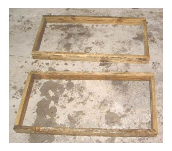
The finished size of these frames should be 48" by 24" on the outside.
