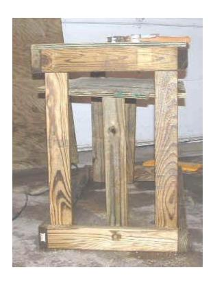
I propped the bottom shelf up with 2 by 4's while I secured the frame that supports it.
